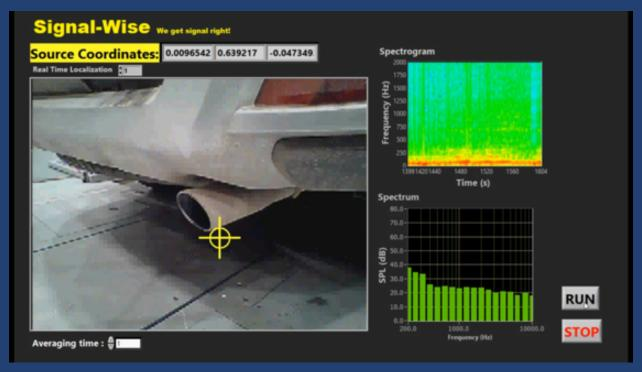
Sound Viewer enables one to locate muffler noise in real time and in post processing. In particular, it enables one to visualize the acoustic pressure and acoustic intensity vector distributions on an arbitrarily shaped surface,<sup>1</sup> and estimate the acoustic power over user-defined surface area.
