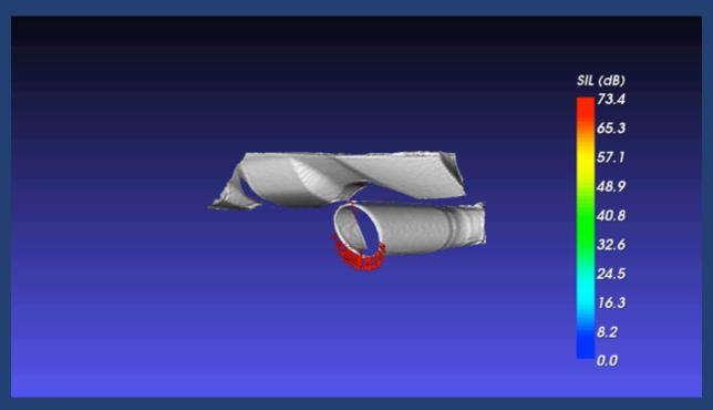
Sound Viewer enables one to visualize the acoustic intensity vector distribution on an arbitrarily shaped surface.
