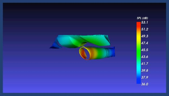
Sound Viewer enables one to visualize the acoustic pressure distribution on an arbitrarily shaped surface.
