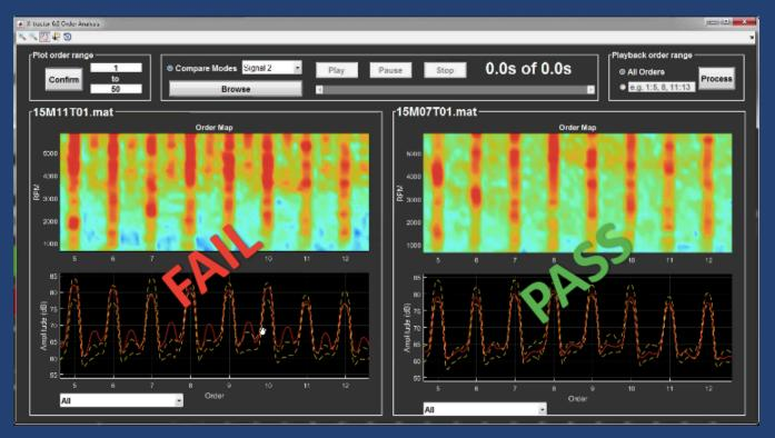
X-tractor enables one to extract target signals in a highly non-ideal environment and discern good products and defective ones. In particular, it can not only detect a defective product, but also reveals what defects are, at which orders and the corresponding speed ranges.
