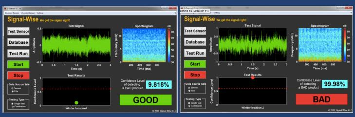
X-tractor enables one to detect a defective product on an assembly line in real time, where the background noise levels on a typical textile factory floor is extremely high.
