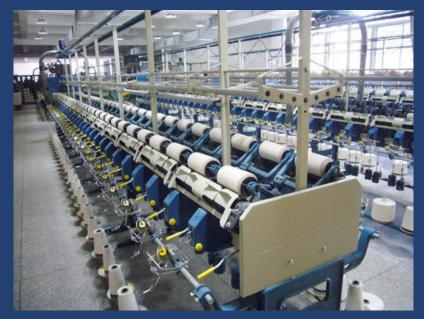
A typical textile factory floor on which winders are lined up one to another at very close distances.
