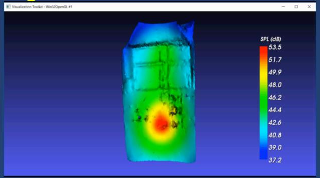
Sound Viewer enables one to visualize the acoustic pressure distribution on an arbitrarily shaped structure.
