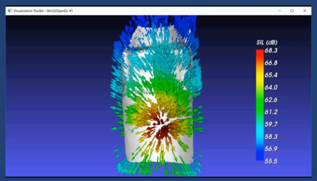
Sound Viewer enables one to visualize the acoustic intensity vectir distribution on an arbitrarily shaped structure.
