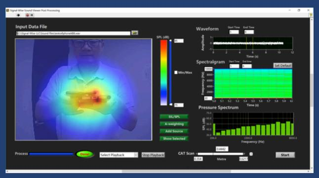
Two cell phones stacked on top of each other with tiny little offset in depth that were producing broadband signals were identified.
