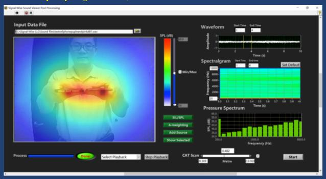
Two side-by-side cell phones that were producing broadband signals were clearly identified.
