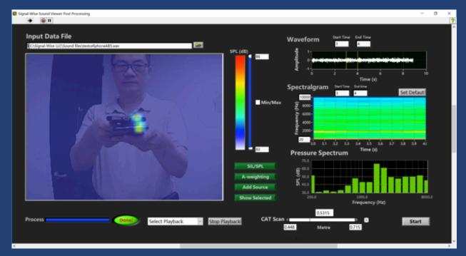
Two cell phones stacked on top of each other that were producing broadband signals were clearly identified.
