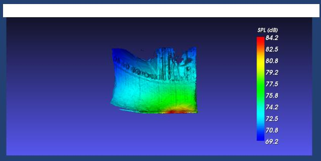
Sound Viewer enables one to visualize the acoustic pressure distribution on an arbitrarily shaped surface.
