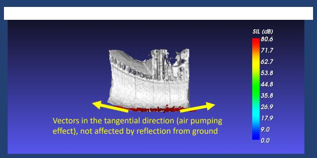
Sound Viewer enables one to visualize the acoustic intensity vector distribution on an arbitrarily shaped surface.
