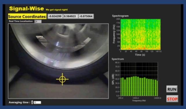
Sound Viewer enables one to locate muffler noise in real time and in post processing. In particular, it allows one to visualize the acoustic pressure and acoustic intensity vector distributions on an arbitrarily shaped surface,<sup>1</sup> and estimate the acoustic power over user-defined surface area.
