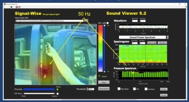
Truck exhaust pipe emitting low frequency noise in 1/3-octave bands centered at 50 Hz was located.
