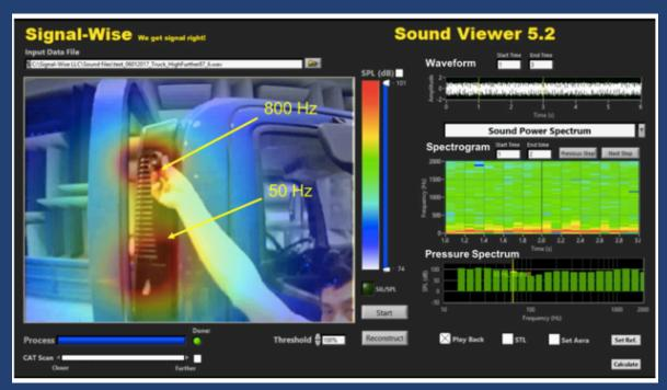
Sound Viewer is capable of locating multiple sound sources in 3D space simultaneously over the frequency range of 20 - 20,000 Hz.
