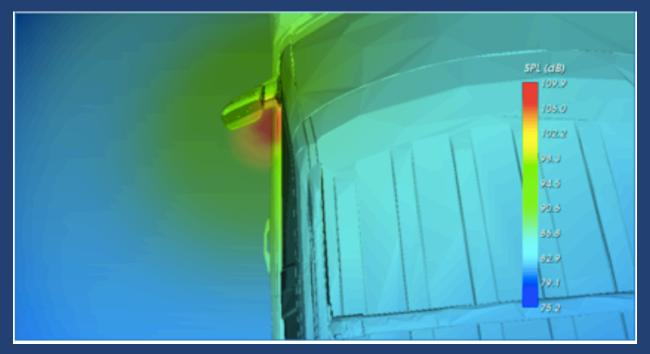
Top view of the acoustic pressure distribution on a horizontal plane behind the rearview mirror, which showed the location where turbulences generated sounds were the strongest.
