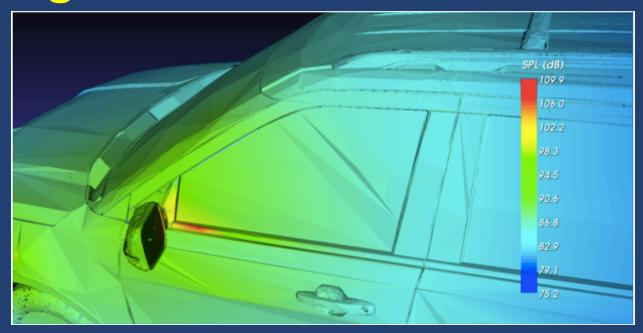
Sound Viewer enables one to acquire the acoustic pressure distribution over the surface of a full-size automobile during the wind tunnel test. In this case, the vehicle was set at zero yaw angle and flow speed was 130 kph. The most dominant flow noise was identified behind the rearview mirror.
