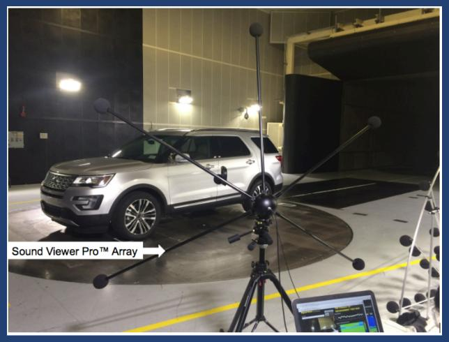
Sound Viewer is capable of reconstructing the acoustic pressure and the time-averaged normal acoustic intensity vector distributions on an arbitrarily shaped object or the entire structure,  $^1$  and is suited for wind tunnel tests to locate multiple sound sources in 3D space simultaneously over the frequency range of 20-20,000 Hz.
