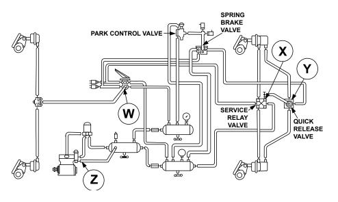
3. The air brake system shown has 120 psi, but the park brake will not release. This could be caused by a leak at:
