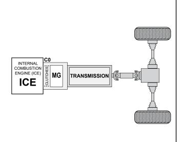
The Type-5 hybrid-drive system uses a power split system like the Type-1. A secondary electric propulsion system is added to provide all-wheel drive.
