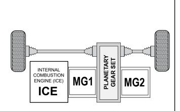
The **Type-2** hybrid-drive is a type of parallel system design.
