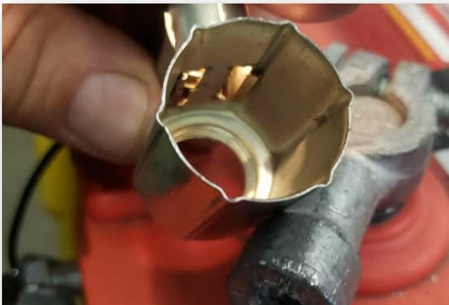
This is the lighter housing and shows how the clips of the light bulb holder attach. This is also where the light from the bulb enters the cigarette lighter housing and it glows in the dash at night when the dash lights are turned on
