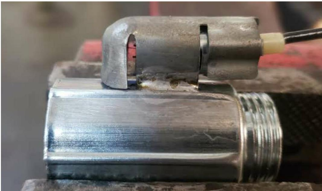
You can see the newly soldered joint. This maintains 100% electrical connection. When installed in the car, this solder is not visible for inspection by the judges.
