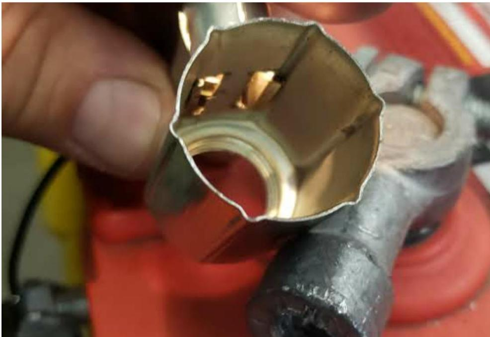
This is the lighter housing and shows how the clips of the light bulb holder attach. This is also where the light from the bulb enters the cigarette lighter housing and it glows in the dash at night when the dash lights are turned on
