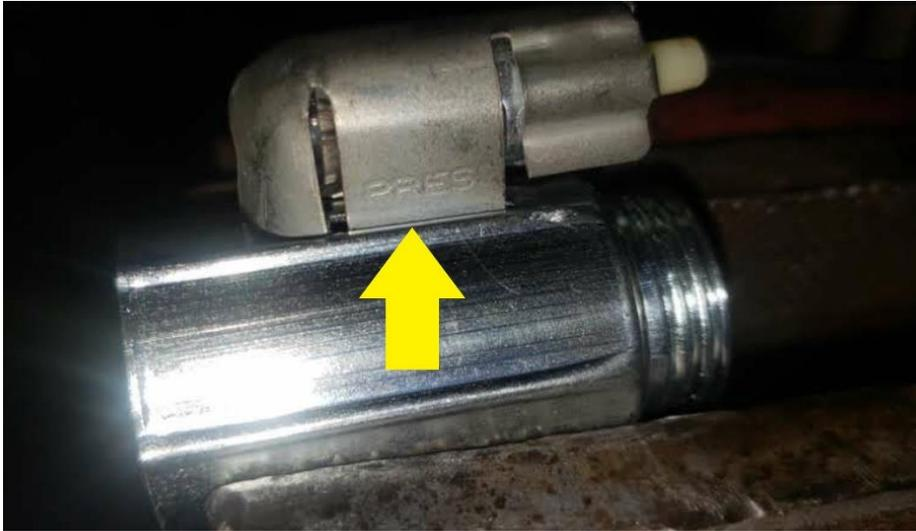
This is where I added solder so that the bulb housing would make good electrical connection. You can see the holder is stamped "PRESS". You pinch both sides and it compresses so it can be removed from the lower housing. After replacing the bulb, the holder would not spring back strong enough to maintain good connection to ground
