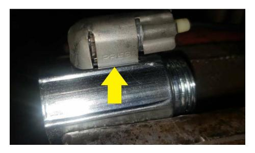
This is where I added solder so that the bulb housing would make good electrical connection. You can see the holder is stamped "PRESS". You pinch both sides and it compresses so it can be removed from the lower housing. After replacing the bulb, the holder would not spring back strong enough to maintain good connection to ground
