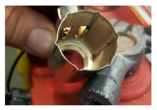
This is the lighter housing and shows how the clips of the light bulb holder attach. This is also were the light from the bulb enters the cigarette lighter housing and it glows in the dash at night when the dash lights are turned on
