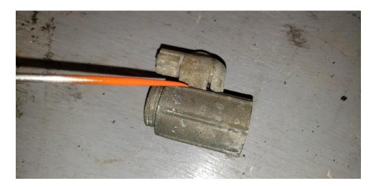
This is the bulb holder on the top and the point it attaches to the housing. This one is dirty and has corrosion but the one we were using was clean. The bulb holder would just lose good contact from time to time causing lack of ground and light bulb going off
