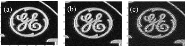
Figure 3. 64 \times 64 image array constructed from a single SE via MR-based Fourier analysis for a GE daily QA phantom portion for (a) f_s=1024 kHz and T_s=8 ms, (b) f_s=256 kHz and T_s=32 ms, and (c) f_s=64 kHz and T_s=128 ms. T2^*_{ij} is randomly assigned for all pixels within the simulated SE, and a constant T2^*_{ij}=40 ms is set during reconstruction to provide partial compensation.
