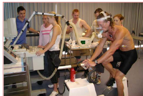
Figure 1. Oxygen uptake monitoring during cycle ergometry for Griffith University exercise science students.
