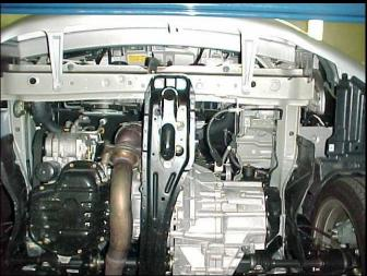
6) Next, remove the 2 bolts that secure the cradle bridge bracket to the radiator support.
