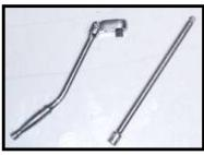
Hotchkis Tuning recommends that this sway bar set be installed by a professional, as the front sway bar can only be removed or installed by detaching the front engine cradle and lowering it from the vehicle!
