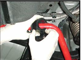
8) Place the provided bushing bracket over the bushing and set the sway bar into it's proper position. Install the provided nut and bolt to secure the bracket to the frame of the vehicle.
