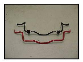
10) Re-install your new Hotchkis sway bar in the same manner as the stock sway bar removal. Install using the included Hotchkis polyurethane bushings and brackets. It's a good idea to install the bushings and brackets after the bar is in position. Lube the inside of each bushing with the provided grease.
