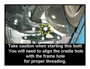
2 – Install the front cradle nuts and torque to **116 ft-lbs**.
