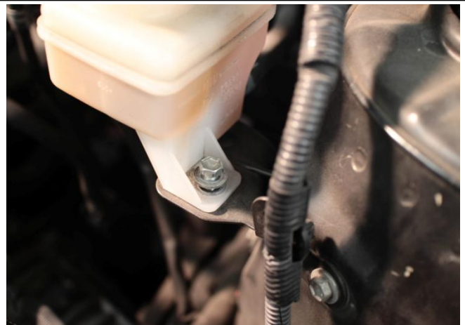
18. Loosen and remove the bolt from the brake fluid reservoir.
