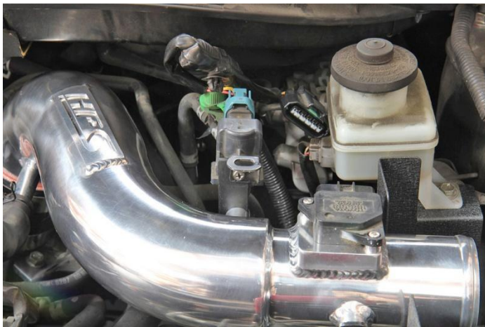
27. Re-using the factory screw, re-install the EVAP sensor onto the sensor bracket along with the factory harness bracket.
