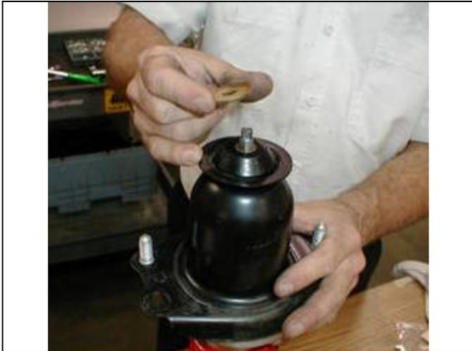
(m) Install a 3/8-24 locknut and cup washer on the shock shaft.
