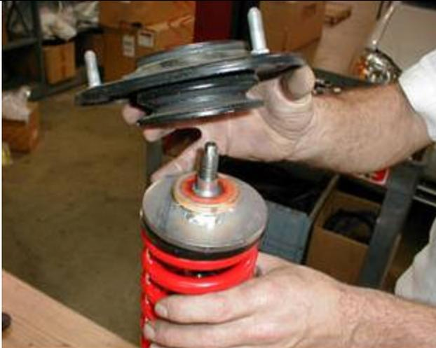
(h) Place the factory front suspension support assembly over the upper bearing adaptor until it is seated on the dust seal.
