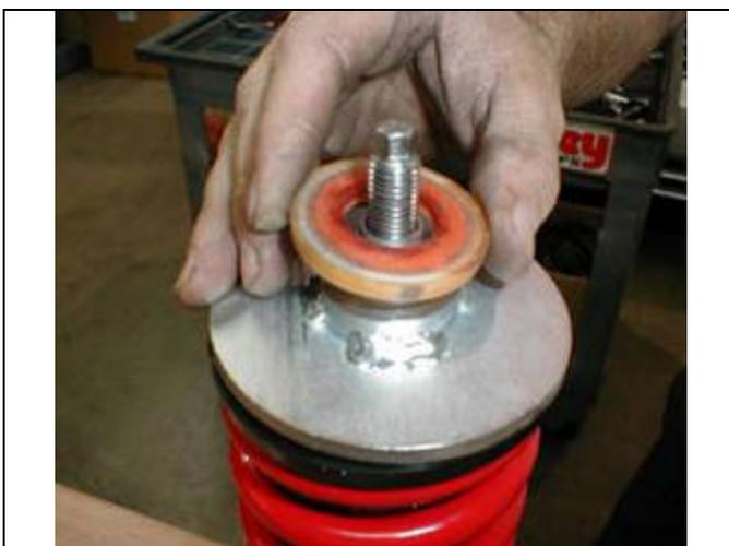
(g) Install the factory front suspension support dust seal over the protrusion on the top of the upper bearing adaptor.
