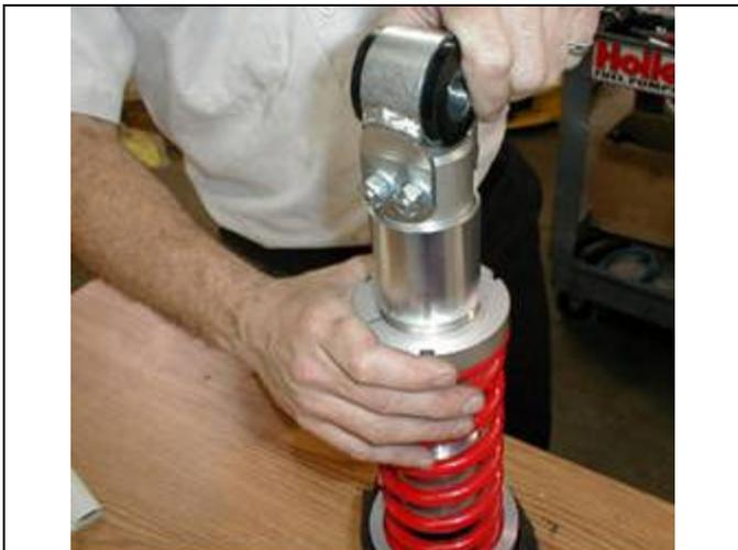
(n) Apply a pre-load to the spring by turning the spring perch so that  $\frac{3}{4}$ " or 20 mm of threads are showing below the spring perch.
