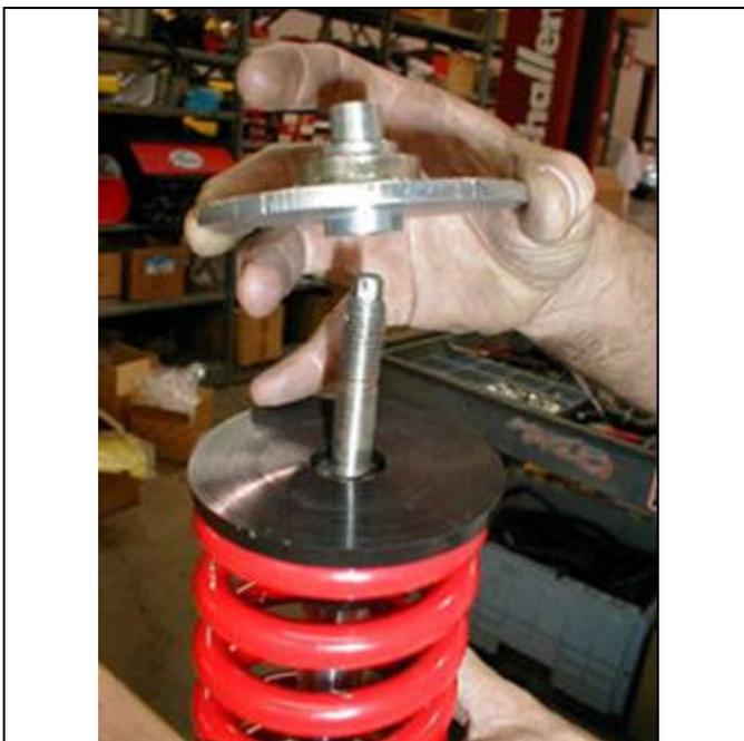
(e) Place the coil spring on the TRD shock with the bump stop at the top.
