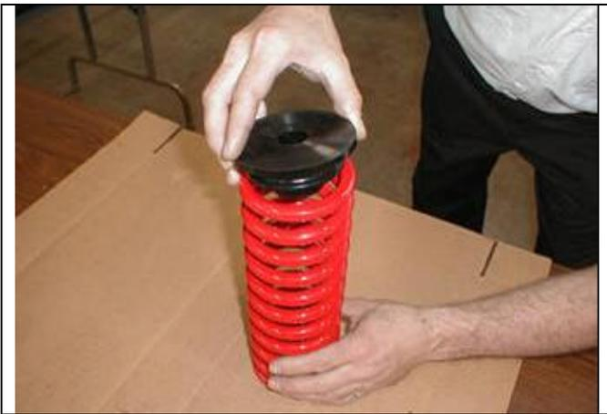
(d) Thread a bump stop/isolator on one end of a front coil spring.
