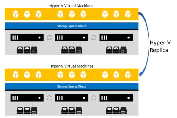
With Hyper-V Replica, the replication is taken care of by Hyper-V. When you first enable a virtual machine for replication, there are three choices for how you wish the initial copy to be sent to the corresponding replica cluster(s).
