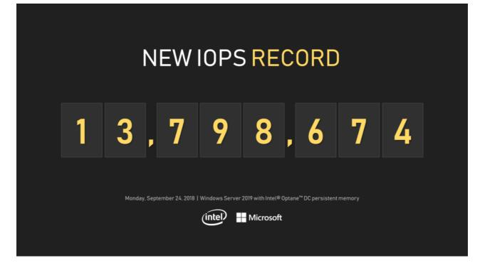
If you watch the video closely, you'll notice that what's even more jaw-dropping is the latency. Even at over 13.7 M IOPS, the file system in Windows is reporting latency that's consistently less than 40 µs! (That's the symbol for microseconds, one-millionth of a second.) This speed is an order of magnitude faster than what typical all-flash vendors proudly advertise today.
