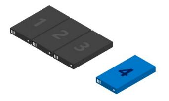
With four servers, you can use dual parity, also commonly called erasure coding (compare to distributed RAID-6). This provides the same fault tolerance as three-way mirroring, but with better storage efficiency. To learn more, see Fault tolerance and storage efficiency.
