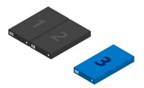
With two servers, you can only create two-way mirrored volumes (compare with distributed RAID-1). With three servers, you can create three-way mirrored volumes for better fault tolerance. We recommend using three-way mirroring whenever possible.
