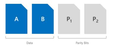
The storage efficiency of dual parity increases the more hardware fault domains you have, from 50% up to 80%. For example, at seven (with Storage Spaces Direct, that means seven servers) the efficiency jumps to 66.7% – to store 4 TB of data, you need just 6 TB of physical storage capacity.
