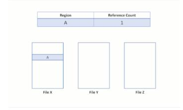
By keeping a reference count for each logical cluster, ReFS doesn't break the isolation between files: writes to shared regions trigger an allocate-on-write mechanism, where ReFS allocates a new region for the incoming write. This mechanism preserves the integrity of the shared logical clusters.
