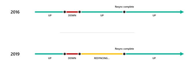
By showing the overall storage resync progress, you can accurately know how much data is out of sync and whether your system is making forward progress. When you open Windows Admin Center and go to the *Dashboard*, you will see the new alert as follows:
