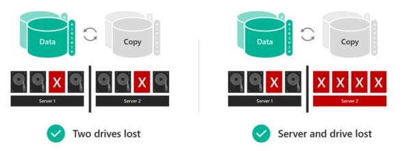
The trade-off is that nested resiliency has **lower capacity efficiency than classic two-way mirroring**, meaning you get slightly less usable space. For details, see the Capacity efficiency section below.
