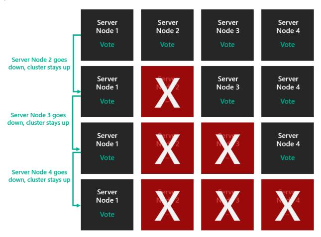
The above scenario applies to a general cluster that doesn't have Storage Spaces Direct enabled. However, when Storage Spaces Direct is enabled, the cluster can only support two node failures. This is explained more in the pool quorum section.
