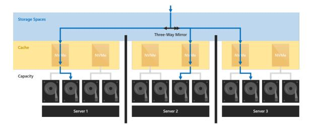
For example, when using three-way mirroring, three copies of any data are written to different servers, where they land in cache. Regardless of whether they are later de-staged or not, three copies will always exist.
