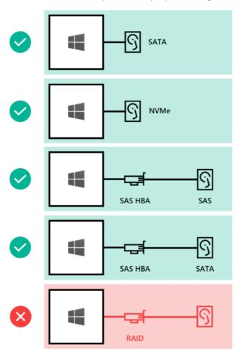
Drives can be internal to the server, or in an external enclosure that is connected to just one server. SCSI Enclosure Services (SES) is required for slot mapping and identification. Each external enclosure must present a unique identifier (Unique ID).
