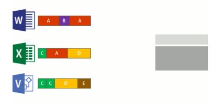
5. Replace the original file stream of now optimized files with a reparse point to the chunk store.
