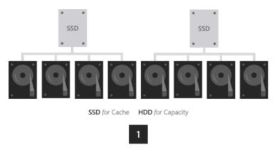
1. **SSD** + **HDD**. The SSDs will cache reads and writes, to absorb bursts and provide SSD-like write performance, with optimized de-staging later to the HDDs.
