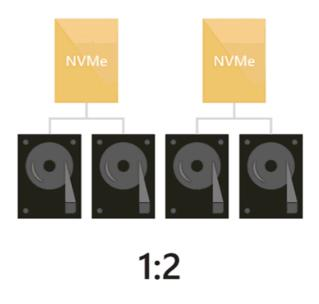
We recommend making the number of capacity drives a multiple of the number of cache drives, for symmetry. For example, if you have 4 cache drives, you will experience more even performance with 8 capacity drives (1:2 ratio) than with 7 or 9.
