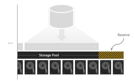
For example, if you have 2 servers and you are using 1 TB capacity drives, set aside  $2 \times 1 = 2$  TB of the pool as reserve. If you have 3 servers and 1 TB capacity drives, set aside  $3 \times 1 = 3$  TB as reserve. If you have 4 or more servers and 1 TB capacity drives, set aside  $4 \times 1 = 4$  TB as reserve.
