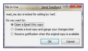
DFSR does have a mechanism for locked files, but it is only within the server's own context. DFSR will not replicate a file in or out if its local copy has an exclusive lock. But this doesn't prevent anyone on another server from modifying the file.
