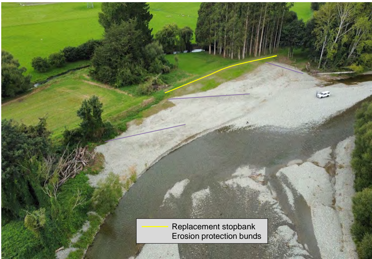
Figure 8-32: Waihi at Hawke Rd Site A following completion of stopbank repairs and installation of erosion protection bunds 23/2/2022
