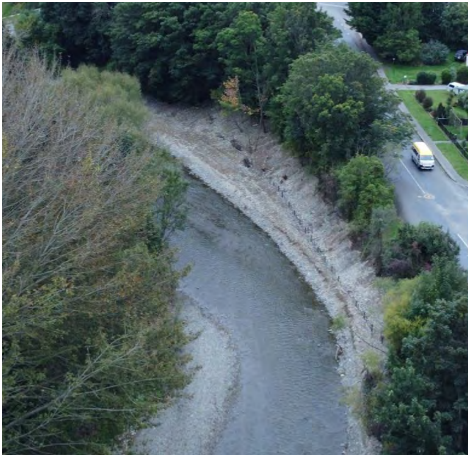
Figure 9-14: Waihi at SH79, Geraldine TLB downstream of bridge. Aerial view looking upstream - completed Heyman Fence repair. March 2022.
