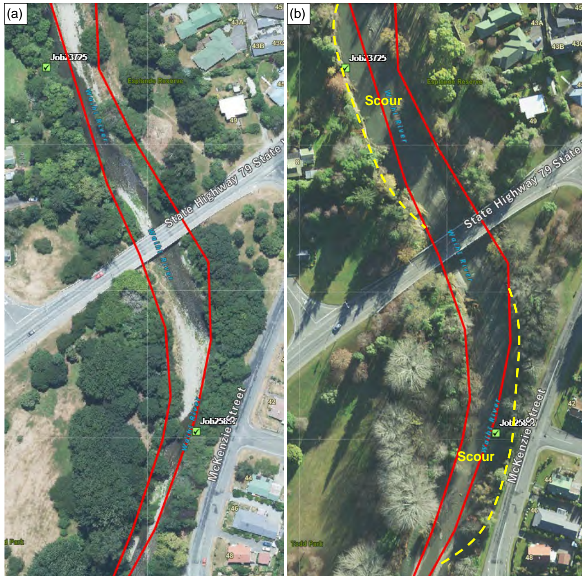
Figure 9-9: Waihi at SH79, Geraldine: (a) aerial view prior to flood, (b) post-flood aerial showing extent of tree edge protection lost.
