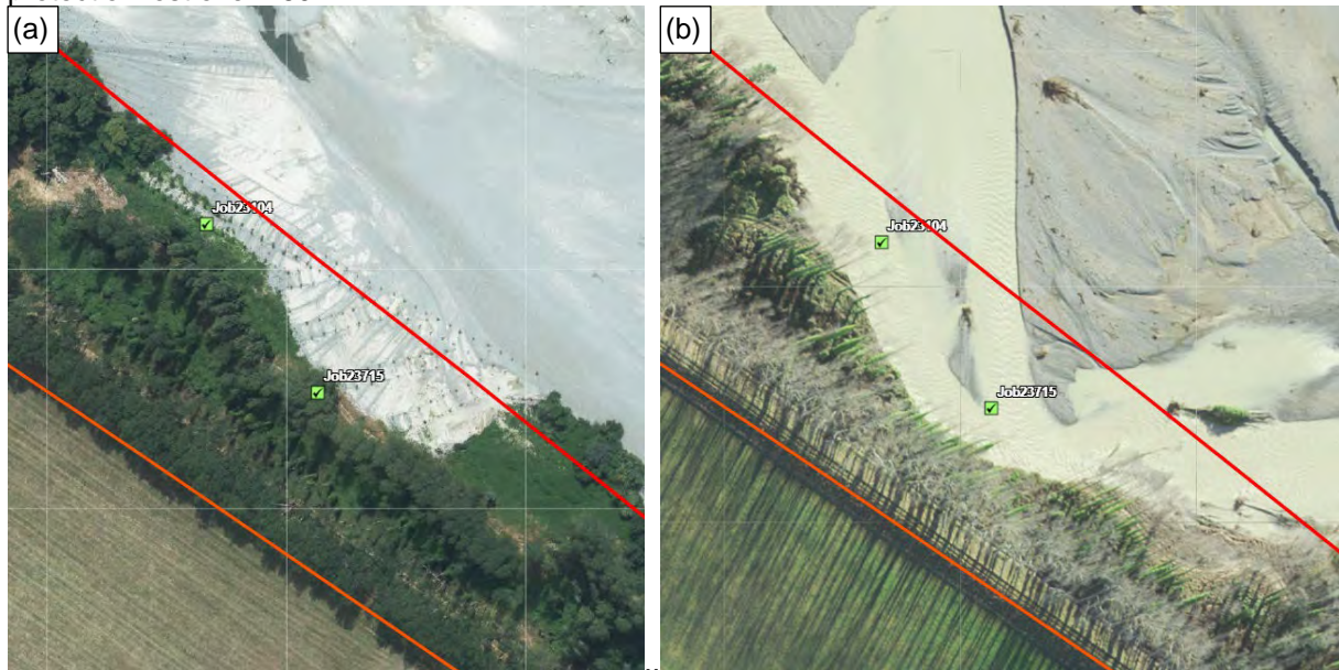
Figure 9-5: Orari at racecourse: (a) aerial view prior to flood, (b) post-flood aerial showing extend of tree edge protection lost.
