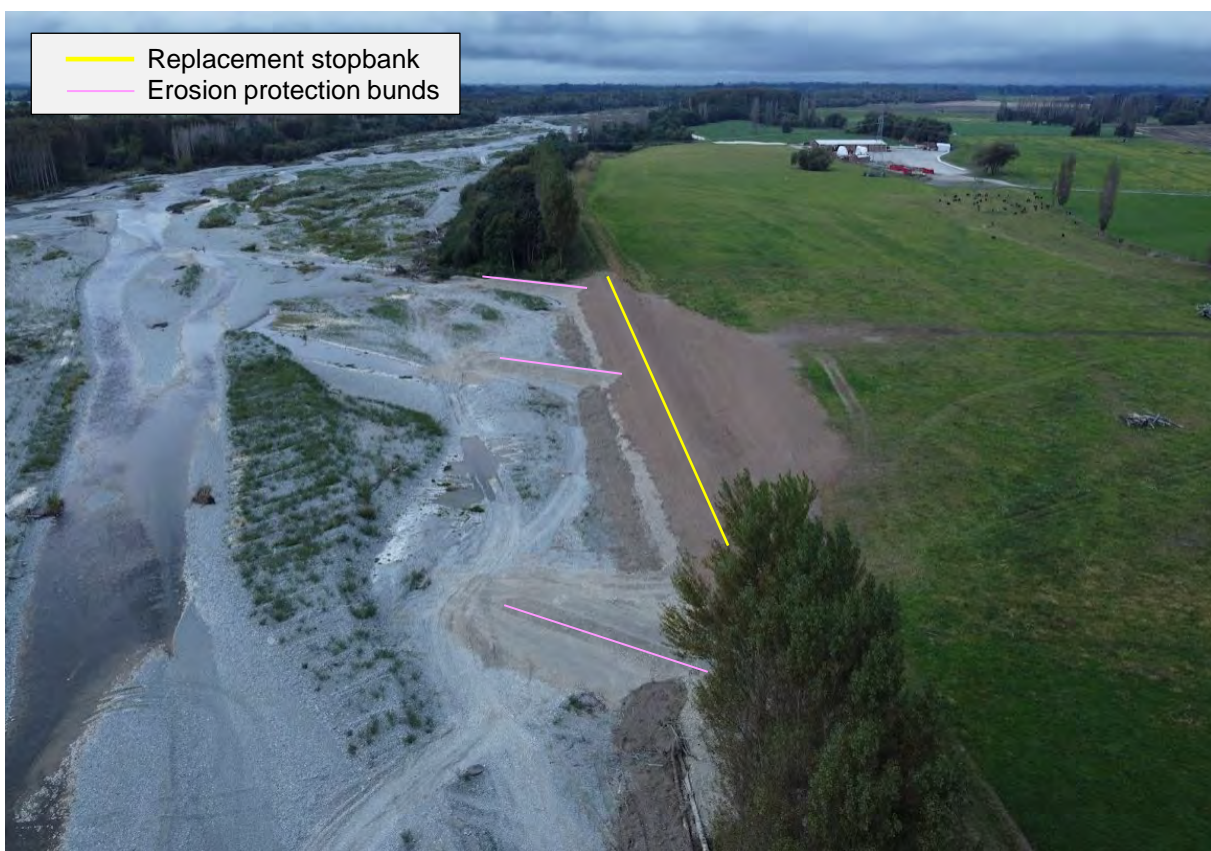
Figure 8-25: Orari at SH7 following completion of stopbank and erosion protection bund works 16/3/2022.
