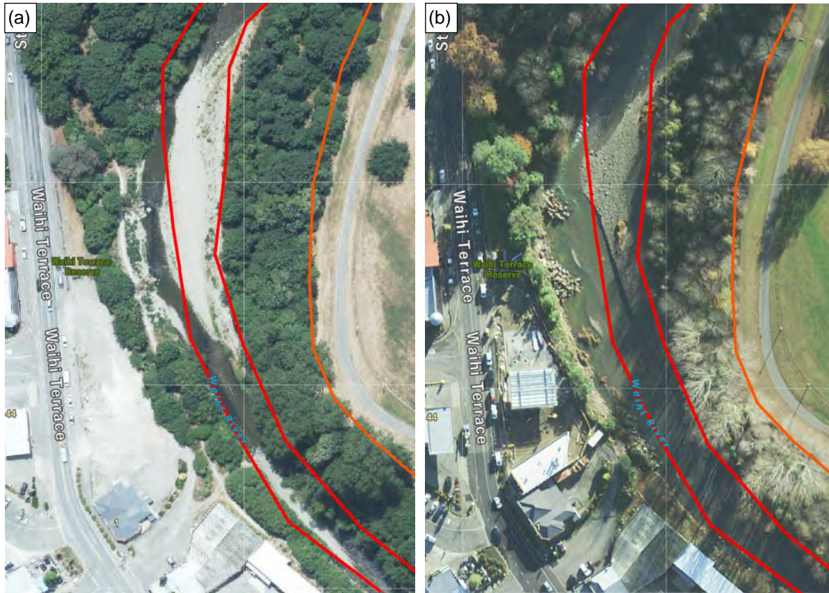
Figure 9-15: Waihi at Geraldine, NPD: (a) aerial view prior to flood, (b) post-flood aerial showing extent of tree edge protection lost.
