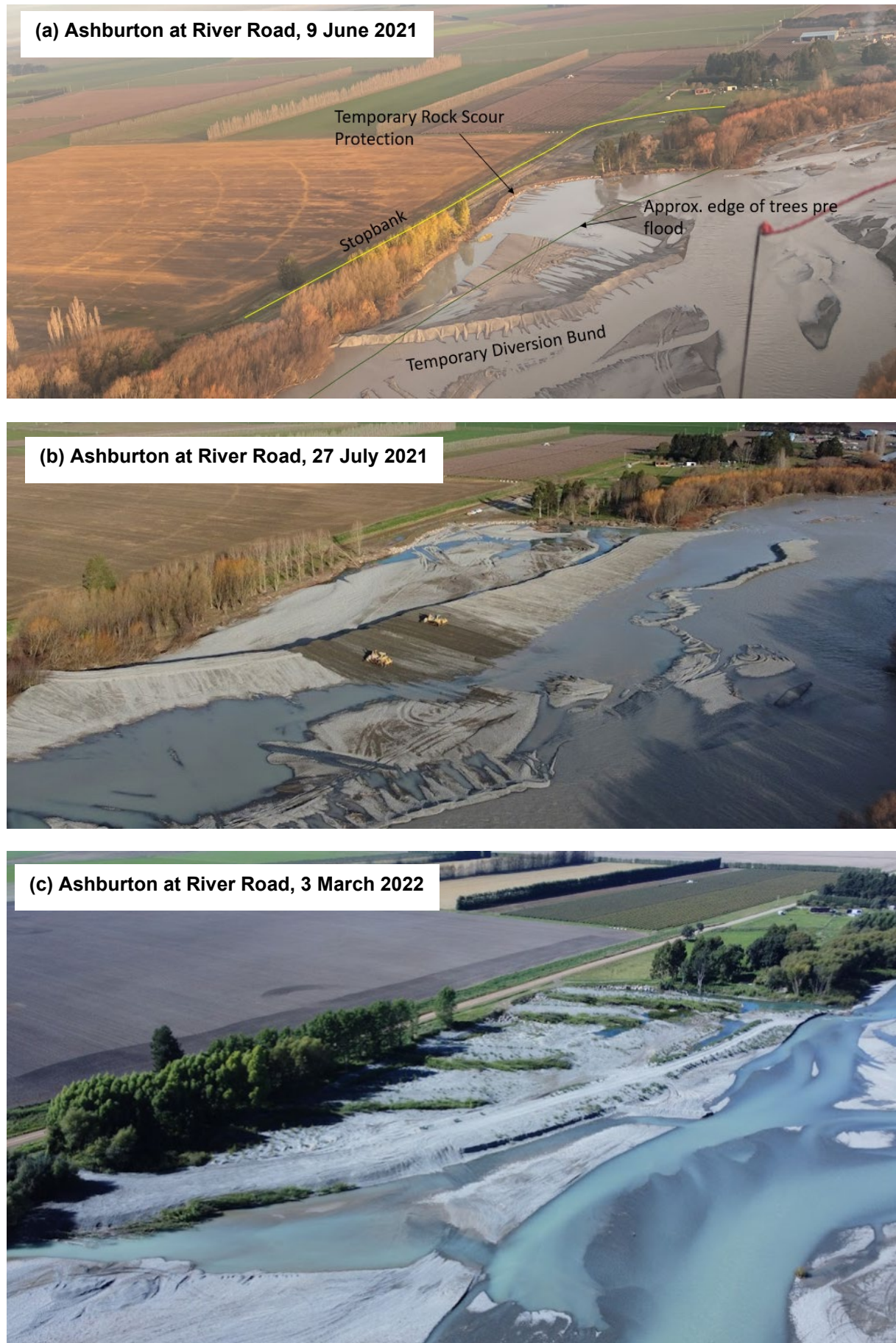
Figure B-5: Ashburton at River Road sequence of flood damage repairs.
