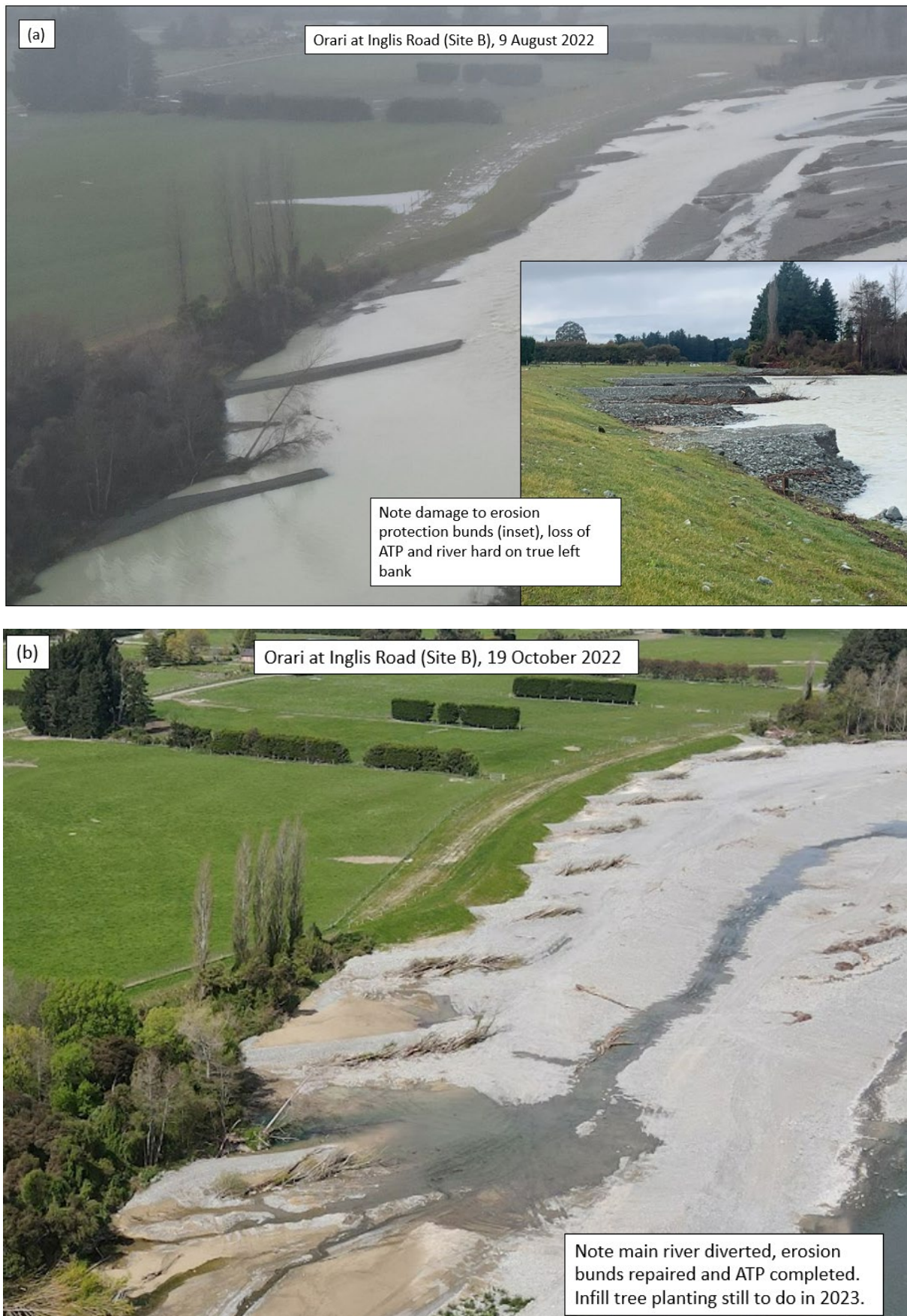
Figure A-6: Orari at Inglis Road, Site B: (a) damage to erosion protection bunds July/Aug 2022, (b) erosion bunds repaired and ATP complete, October 2022.
