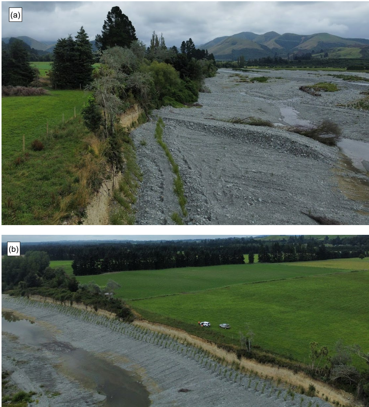
Figure A-8: Orari at Peacocks showing rows of infill planting along edge of eroded high berm in January 2022, (a) looking upstream, (b) looking downstream.
