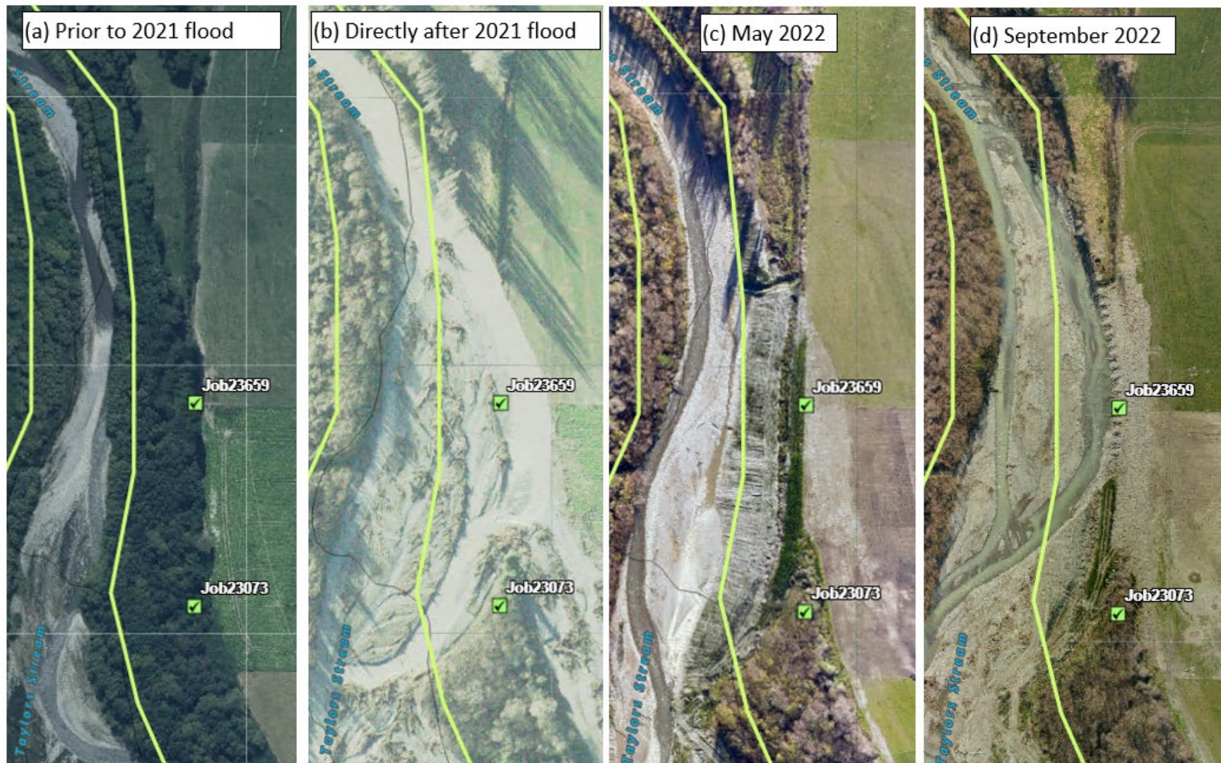
Figure A-14: Taylor's Stream showing (a) pre-flood light anchored bank protection, (b) loss of LABP and flood breakout, (c) bunding and treed trees to stabilise bank, May 2022, and (d) more substantial treed trees, September 2022.
