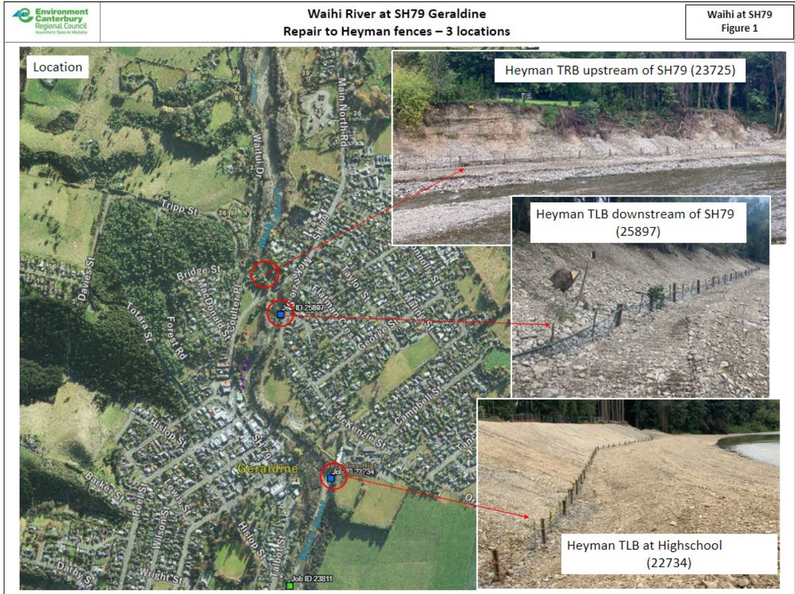
Figure C-7: Waihi at Geraldine, completed Heyman fences following 2021 flood damage.
