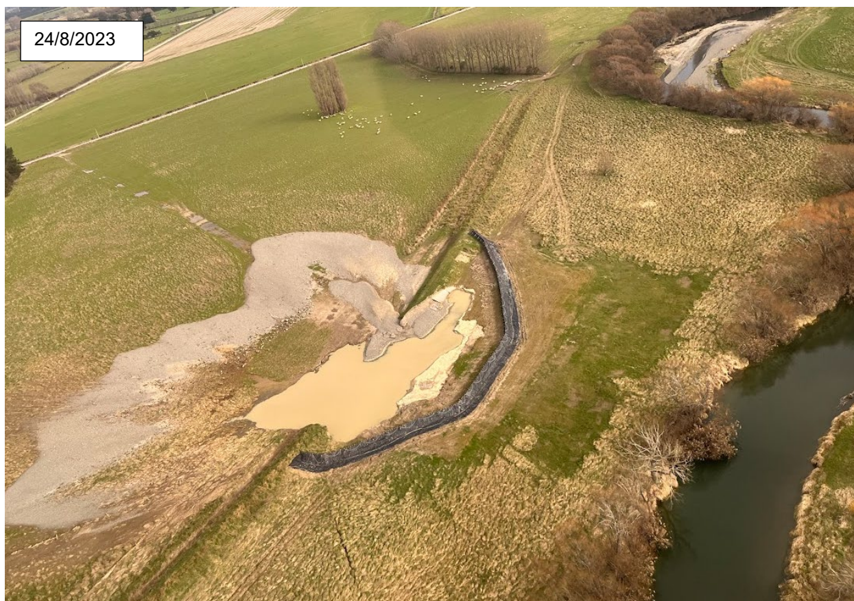
Figure A-10: Selwyn River failure of stopbank and temporary flood barrier. 24/8/2023.
