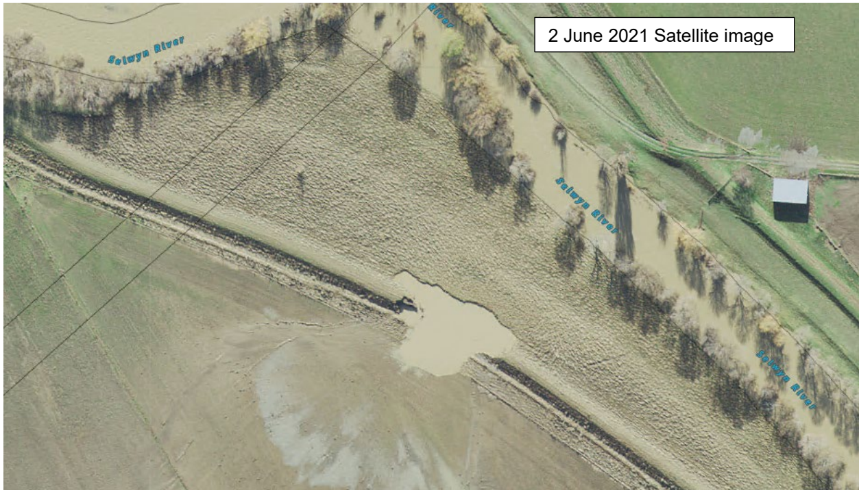
Figure A-8: Selwyn River stopbank breach immediately after 2021 flood.
