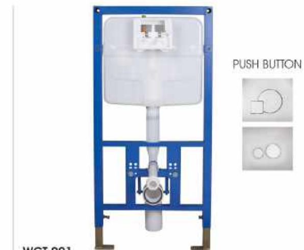
WCT-001 CONCEALED TANK WITH FULL FRAME & INTERNAL FITTINGS L 590 W 75 H 1140
