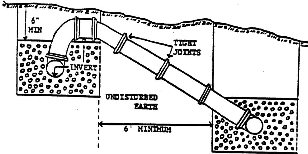
NOTE: Invert of the first relief line must be at least 1 inch lower than invert of the septic tank outlets.
