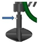
Align lock bolt hole on output shaft
