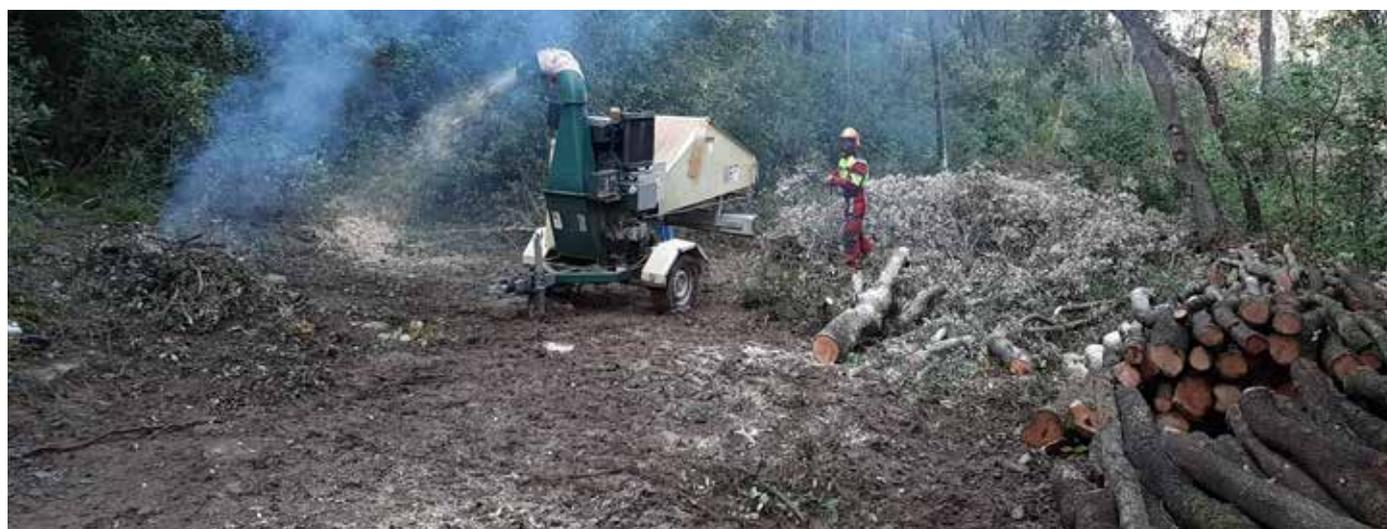
**Figure 1.** Chipping the branches in the field with a shredder to produce BRF. Photo: Montse González, AV Video.
