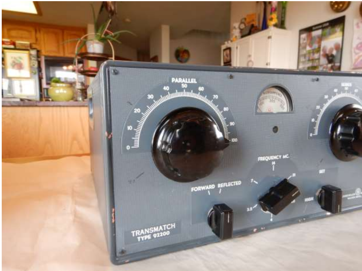
Figure 80: James Millen 92200 Ultimate Transmatch - Front left side. Note the copper where the paint has been chipped
