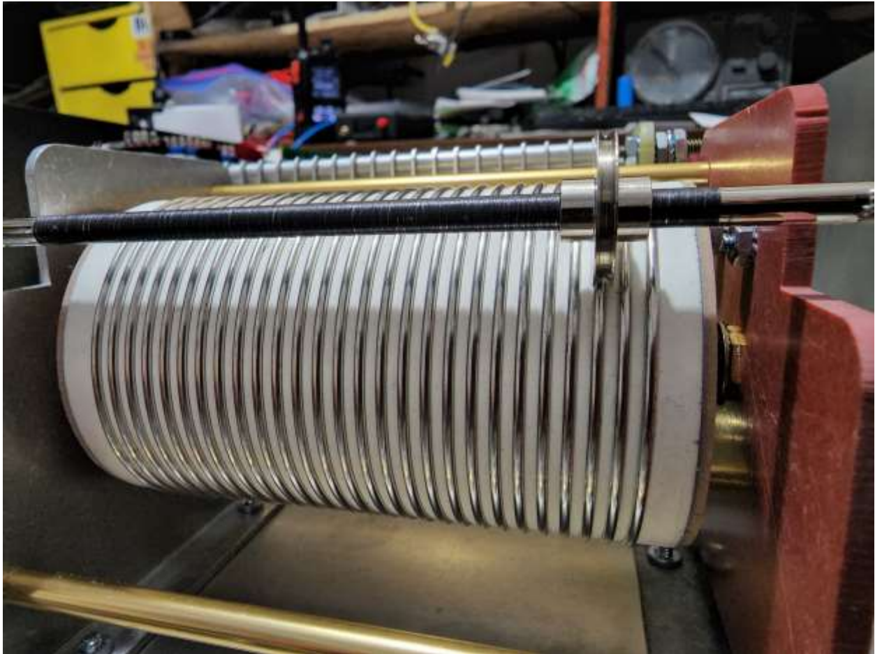
Figure 85: Palstar AT2K - Roller inductor – This is what high quality looks like.
