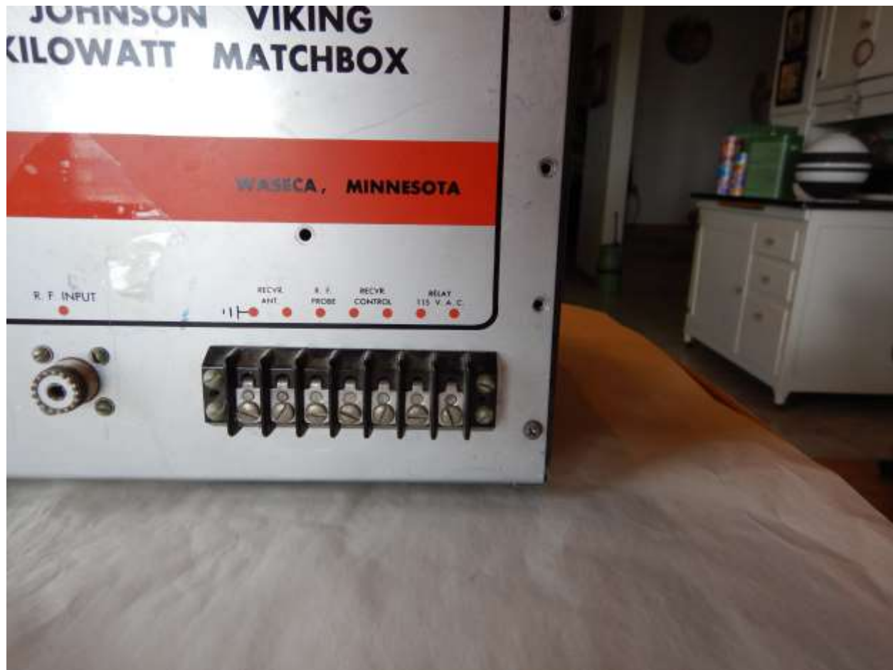
Figure 65: KW Johnson Matchbox - this was for connecting the tuner to the Johnson kilowatt amplifier
