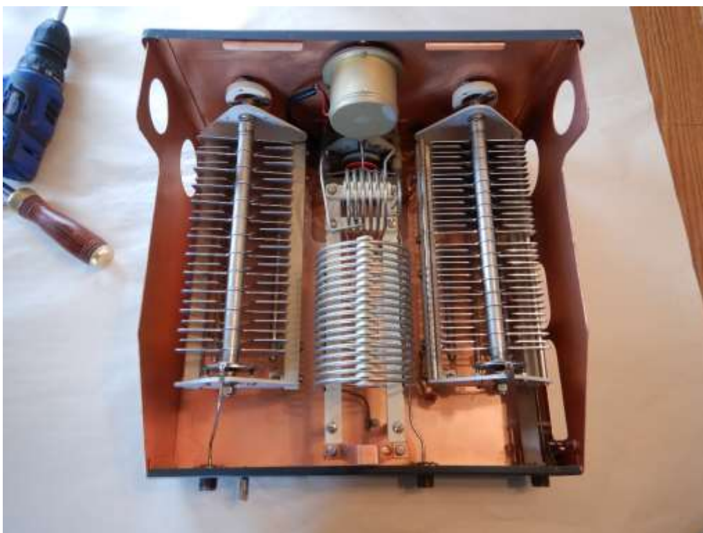
Figure 74: James Millen 92200 Ultimate Transmatch - The case is made completely of copper!
