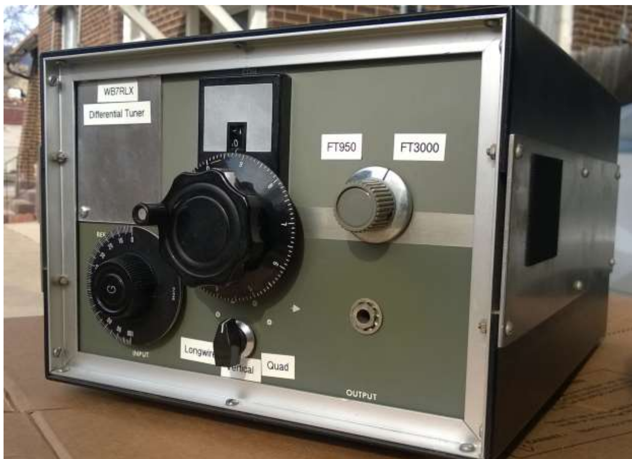
Figure 66: WB7RLX Differential Tuner – Note the unused hole in the front. I'm going to mount a propagation compensator in the unit and locate the control switch there. A note on the six position antenna selector switch: When the switch is pointing above horizontal, as it is in the picture, the tuner is engaged. If the arrow is pointing below the horizontal then the tuner is disengaged.
