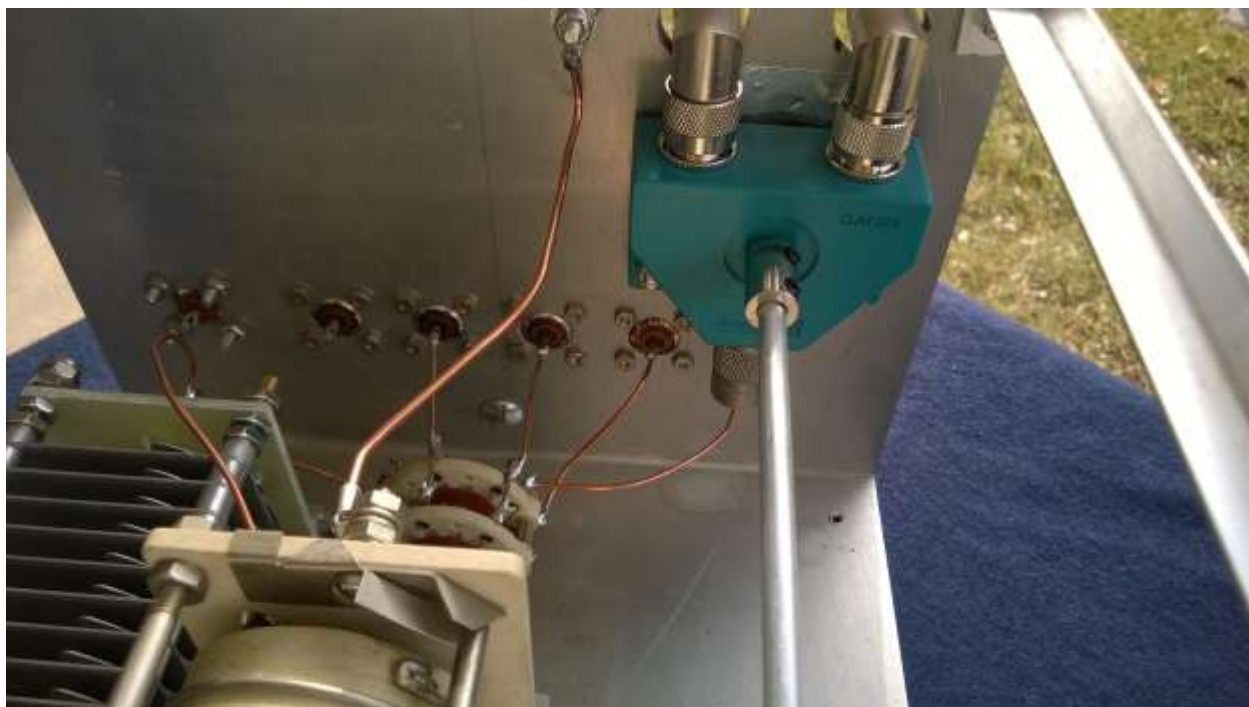
Figure 70: WB7RLX Differential Tuner - looking toward the antenna switch. Note the two ports on the left are not used.
