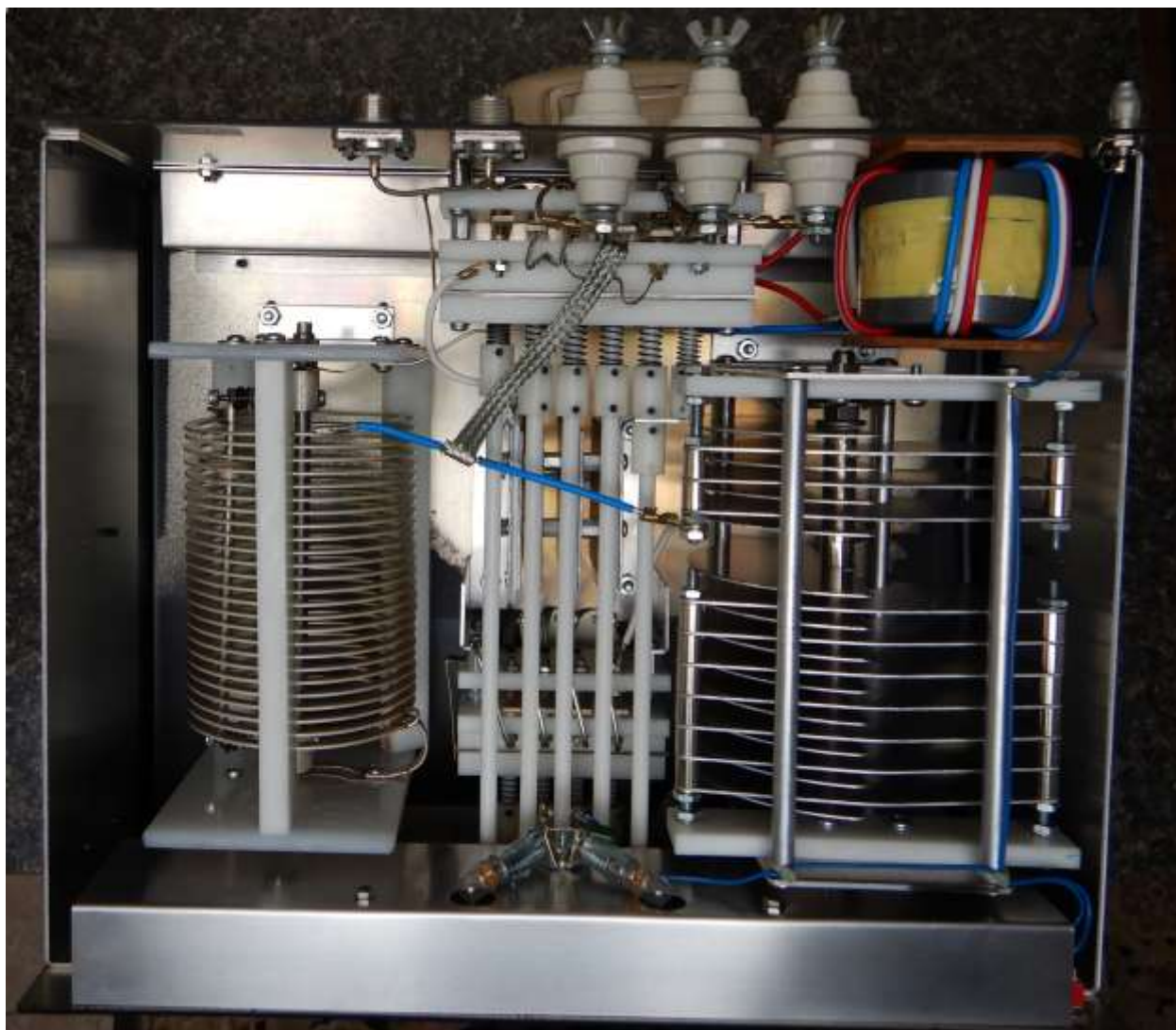
Figure 45: Nye Viking 3KW Tuner - Note the variable capacitor. It's huge! This one of the biggest capacitors I've seen in a tuner. The only other capacitor that is possibly bigger is the one in the Johnson Match Box.
