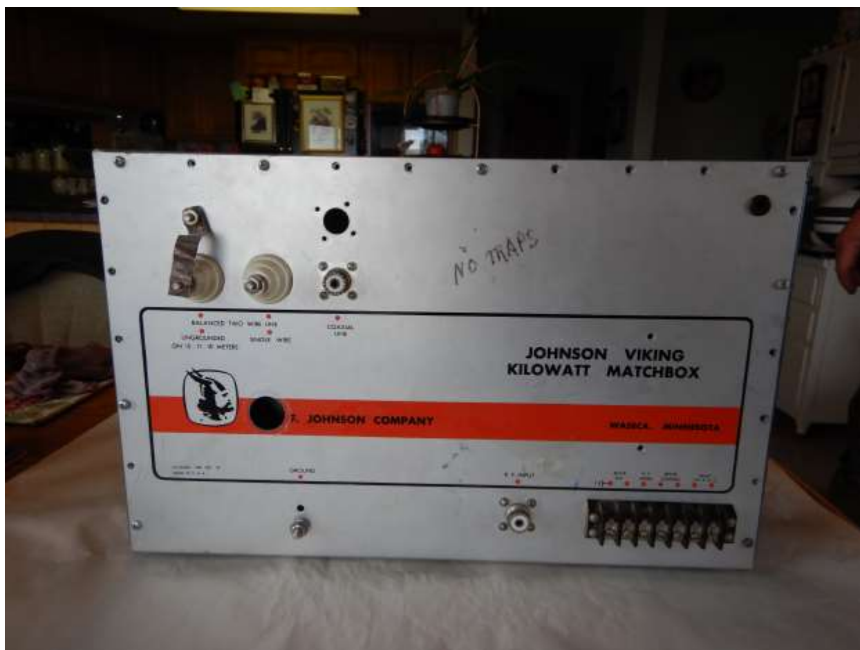
Figure 59: KW Johnson Matchbox - Rear view. Note the extra hole that someone added for an SO-239 socket. The small hole in the top right was for the SWR wire that attached to an external directional coupler.
