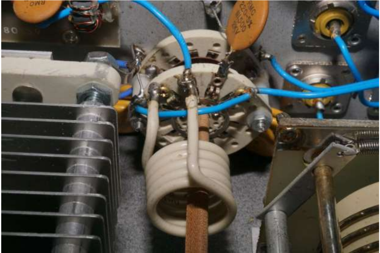
Figure 51: Ten Tec Model 238 - A close look at the rotary switch
