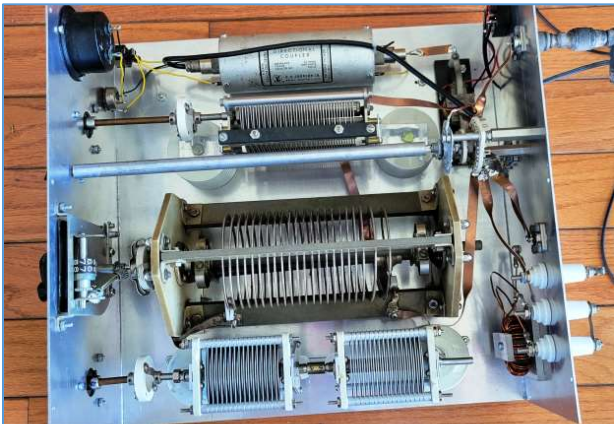
Figure 17: Homebrew Ultimate Transmatch built by John Burger KB0ES. This tuner was built in 1977. Note the use of the interconnecting copper straps and the high quality rotary switch.
