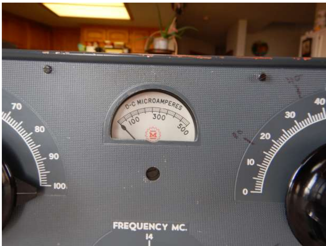
Figure 79: James Millen 92200 Ultimate Transmatch – Power (SWR) Meter. A front panel switch was used to select forward or reflected power.
