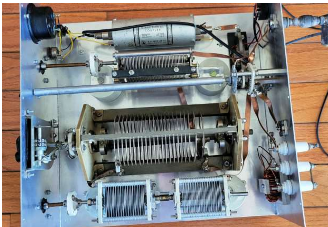
Figure 32: KB0ES Home Brew Ultimate Transmatch. Note the massive inductor and the use of copper strips rather than round copper wire. This is a very well made tuner, one of the best I have seen.
