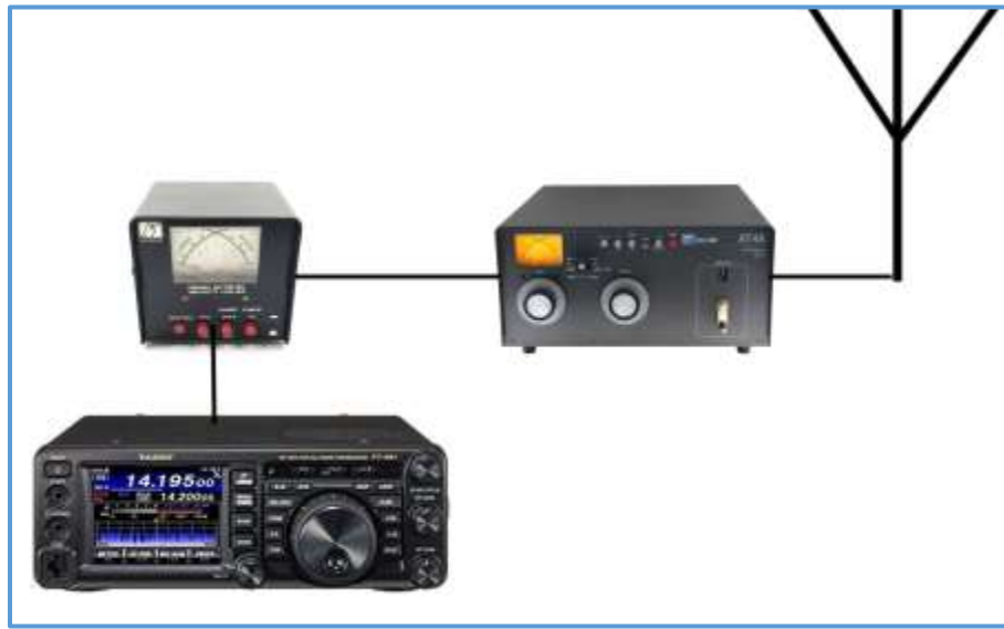
Figure 28: Typical Station Using an External Tuner
