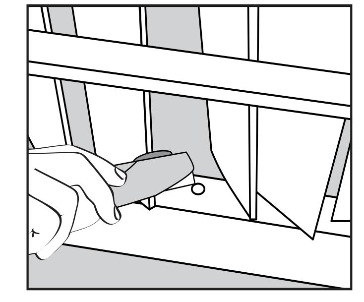
To remove louver, place utility knife blade between louver and panel edge. Lightly tap knife with hammer to cut through louver pin.
