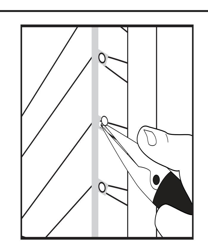
Use needle nose pliers to pry nail out of rear tilt. Also, remove louver pin from other edge of panel.
