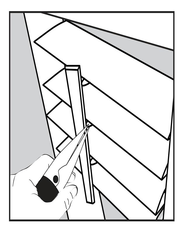
Use needle nose pliers to remove staple from tilt bar.
