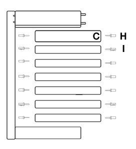
Using a flat surface start inserting the louvers C into your panel assembly ensuring the 1st louver is overlapped by each following louver fitting into the rabbet ends of the top & bottom rail B.
