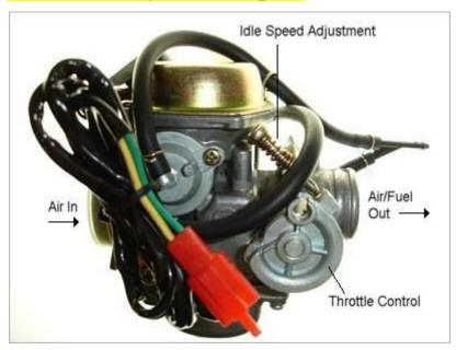
Above is a picture of a typical GY6 engine carburetor and the view is that from the right side of most engine configurations on 50cc Chinese scooters.
