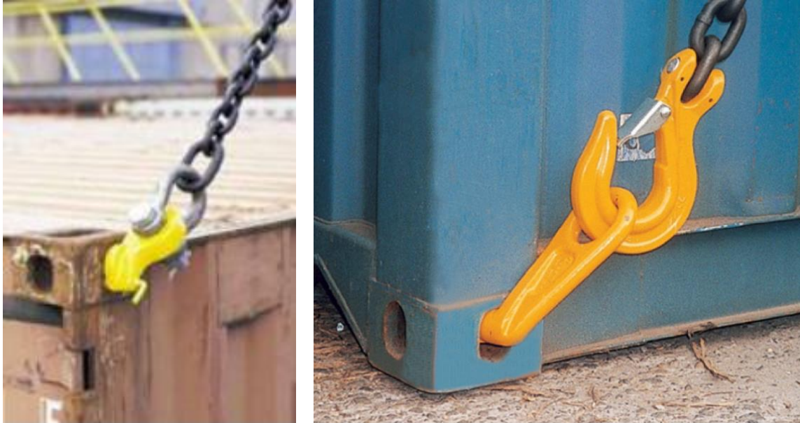
Figure 2: Typical Side Lifting Lugs, showing top and bottom arrangements.
