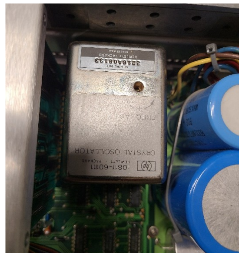
Option Stickers Left, C10 Timebase “Extra” on Right
