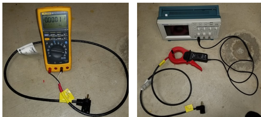
Use with a multimeter (left) and an oscilloscope (right)
