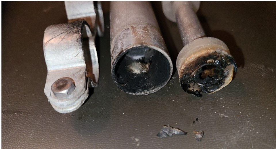
17M Trap Showing the Damage
