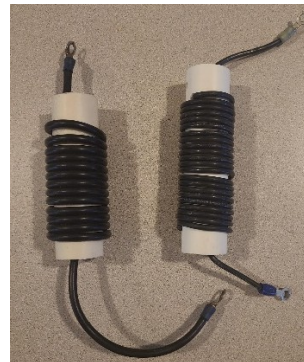
Shunt Coil Match (left), Smith Chart Showing Effects, Two Different Coils
