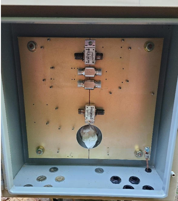
Ground plane with arrestors (left), finished box (right)
