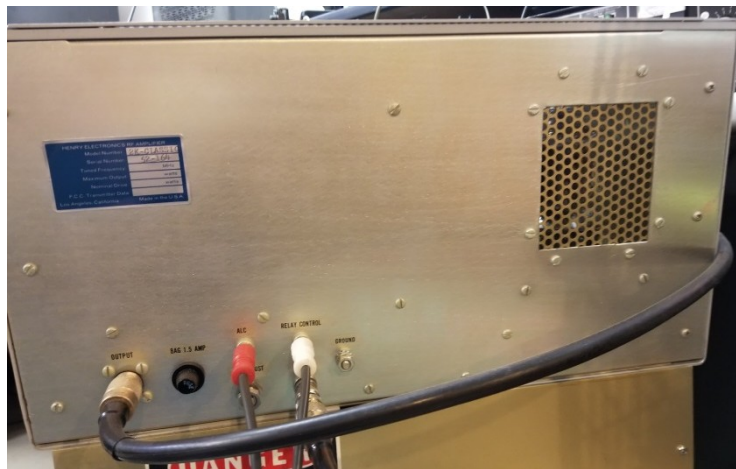
Jumper with a UHF <-> BNC adapter on original Henry rear panel
