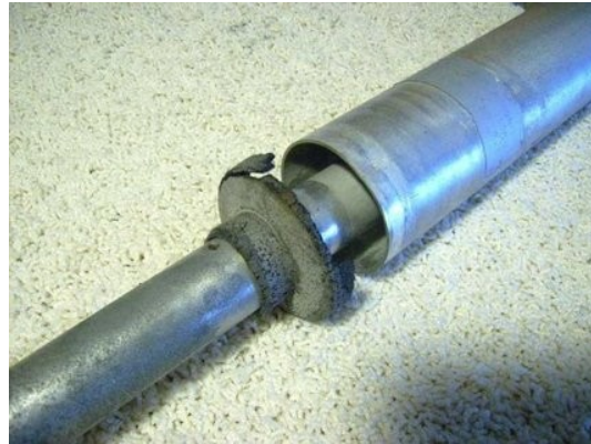
Example of a rotted hy-gain trap seal
