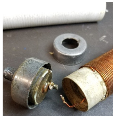
Disassembled antenna (left), and open connection in top coil (right)
