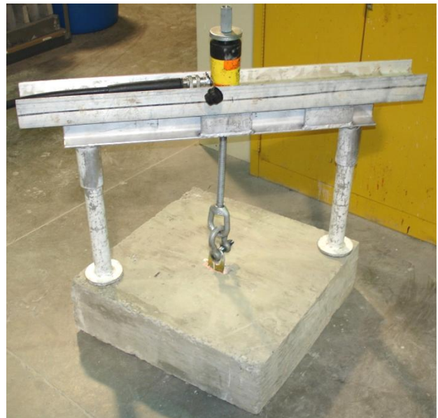
Anchor Tab Mockup in Direct Tension
