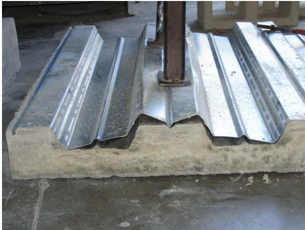
Deformation / separation of metal deck
