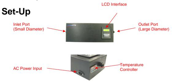
The unit comes prepared and assembled, so no calibration or assembly are required. After unpacking the NDIR, simply attach the inlet to your sample gas line, and the outlet to your vent.
