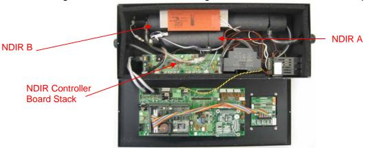
Gain access to the NDIR controller board for the sensor you will be working with. For NDIR A, you will use the top board. For NDIR B, it will be necessary to remove the nuts holding the top board and lift the board out, to gain access to the bottom one.
