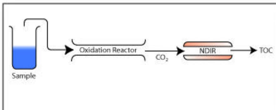
In Total Organic Carbon (TOC) analysis, the sample is generally oxidized in a reactor where carbon is directly converted to CO<sub>2</sub> gas and other chemical species are converted to their respective oxides. Thus, the CO<sub>2</sub> detector must be specific to CO<sub>2</sub> gas ONLY, which is in proportion to the carbon present in the sample and provides a direct correlation to TOC.
