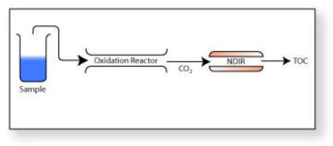
In Total Organic Carbon (TOC) analysis, the sample is generally oxidized in a reactor where carbon is directly converted to  $CO_2$  gas and other chemical species are converted to their respective oxides. Thus, the  $CO_2$  detector must be specific to  $CO_2$  gas <u>ONLY</u>, which is in proportion to the carbon present in the sample and provides a direct correlation to TOC.
