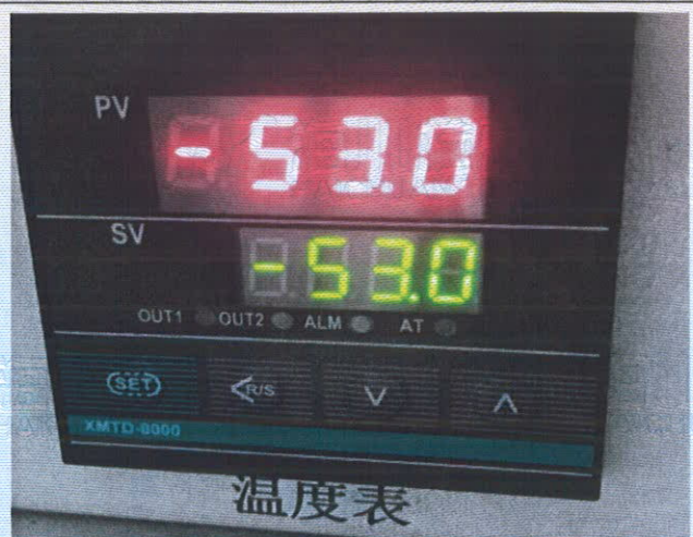
低温测试温度 (-53°C) /Test temperature @ Low temperature (-53°C)
