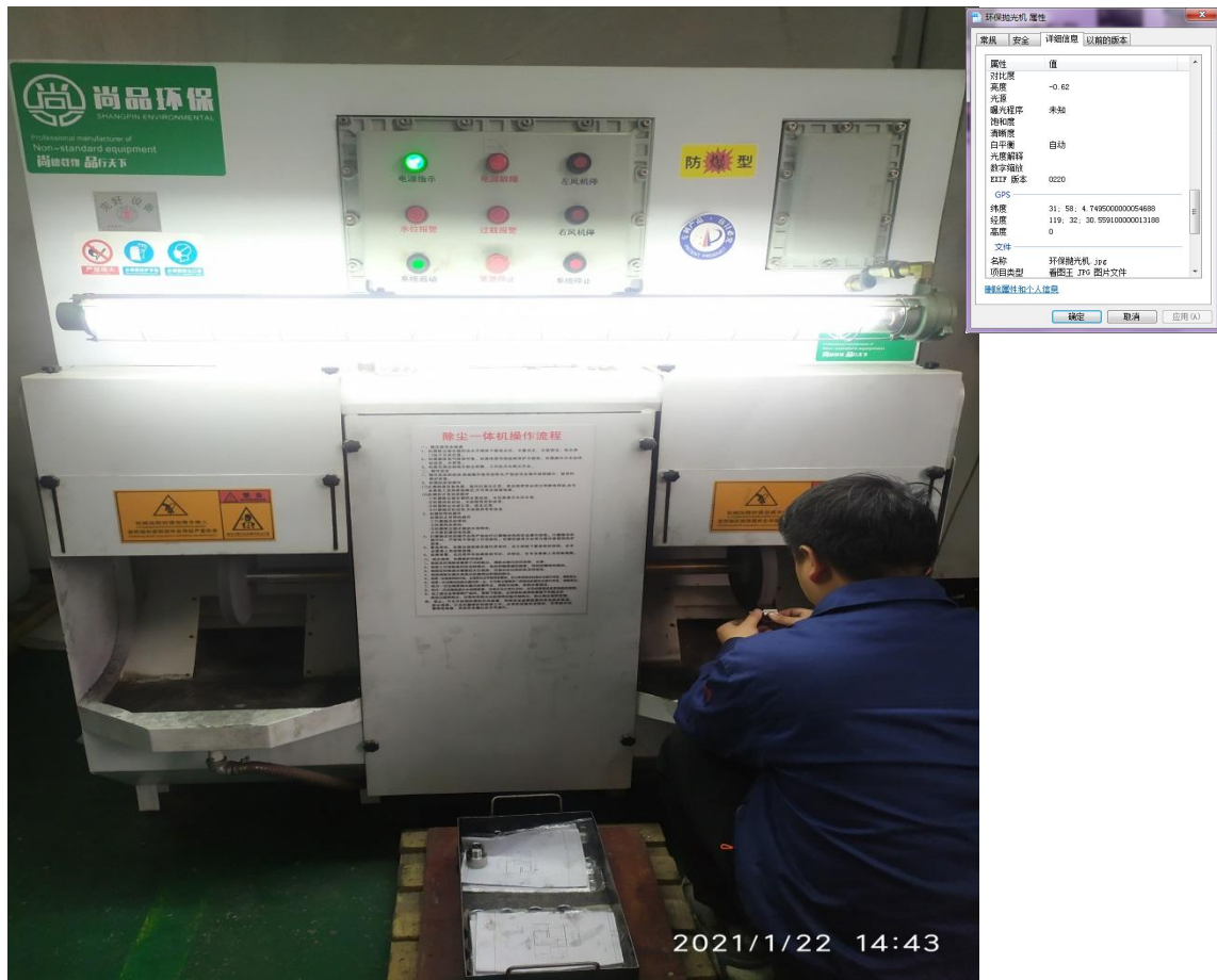
Explosion-proof composite eco-friendly wet dust removal integrated machine
