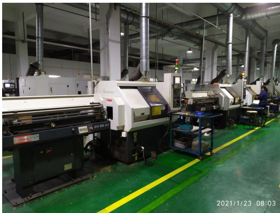
CNC core walker-ferrule processing
