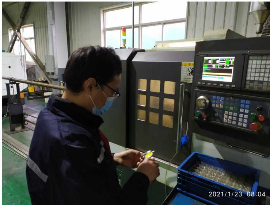
CNC core walker-ferrule processing
