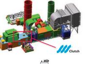
LOAD CENTER: Peaking gas turbines with SSS® Clutches provide quick start real power as well as synchronous condensing for intermittent renewable resources of energy. SSS<sup>®</sup> Clutches enable generator inertia and reactive power for grid support.
