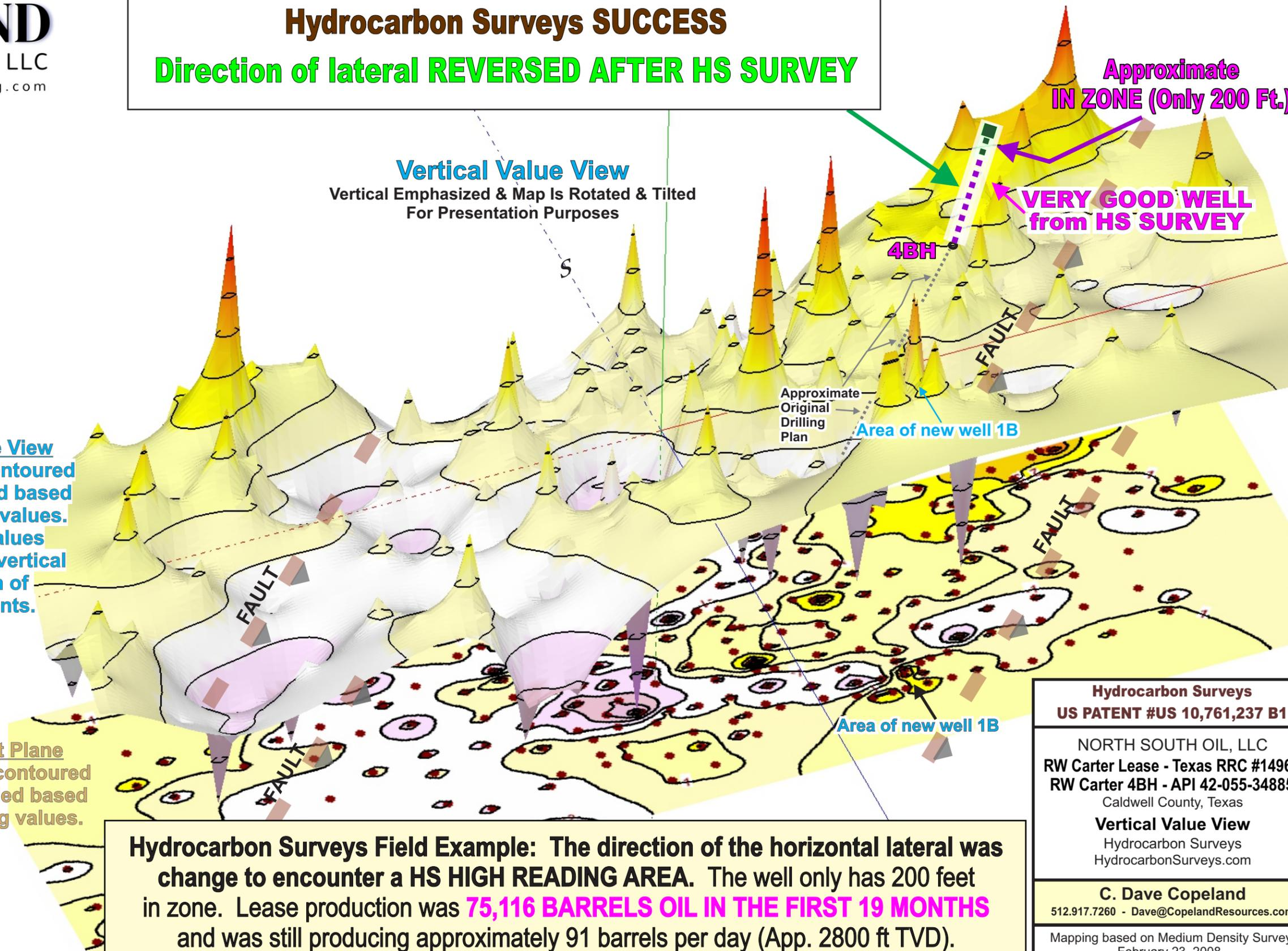
**Hydrocarbon Surveys Field Example: The direction of the horizontal lateral was change to encounter a HS HIGH READING AREA. The well only has 200 feet in zone. Lease production was 75,116 BARRELS OIL IN THE FIRST 19 MONTHS and was still producing approximately 91 barrels per day (App. 2800 ft TVD).**
