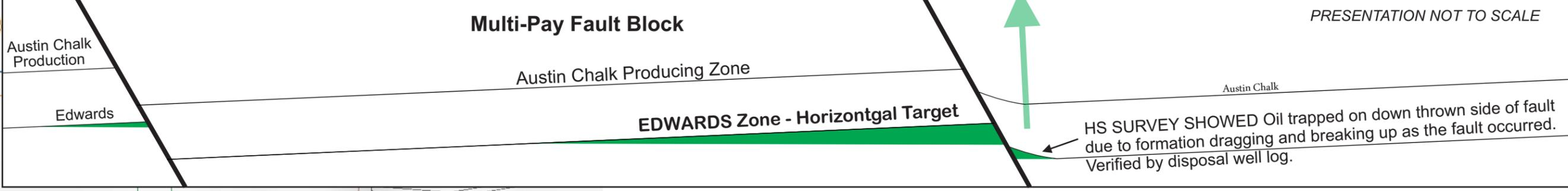
**Hydrocarbon Surveys Field Example: The direction of the horizontal lateral was change to encounter a HS HIGH READING AREA. The well only has 200 feet in zone. Lease production was 75,116 BARRELS OIL IN THE FIRST 19 MONTHS and was still producing approximately 91 barrels per day (App. 2800 ft TVD).**
