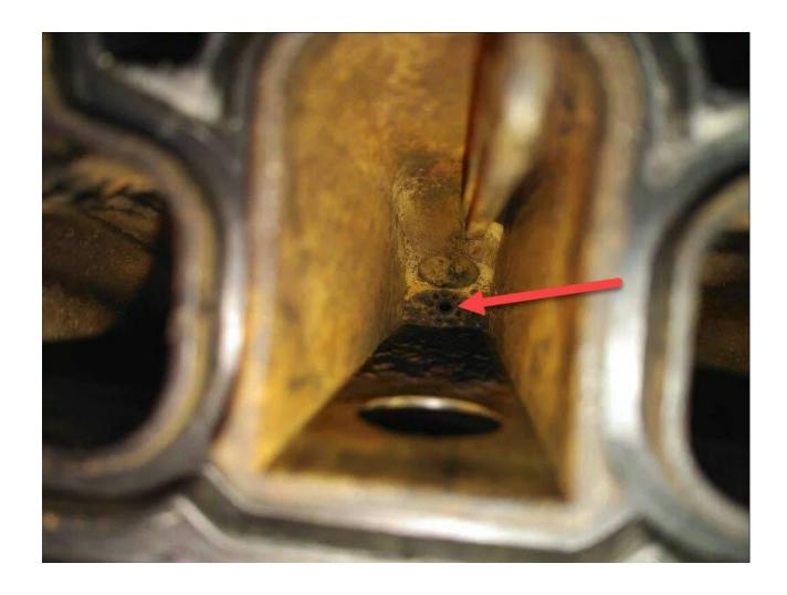
4. Place the washer over the screw, and liberally coat the screw thread with epoxy. The more you can pile on there, the better. Have at least as much as shown below, more if possible.
