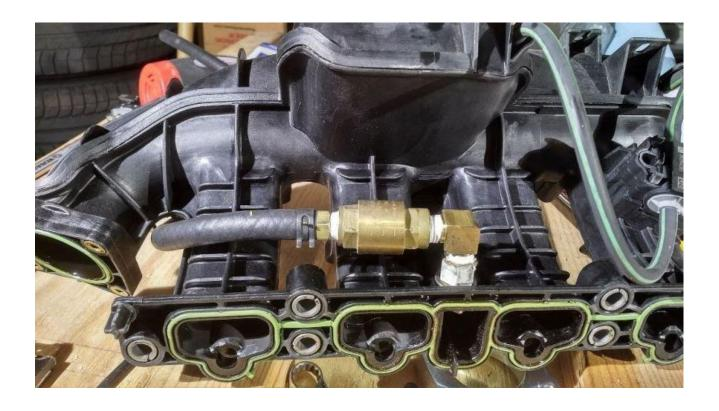
13. Lastly, attach the brake booster tee fitting to the hose in the same fashion as in the last step, and install the fitting on the intake manifold as shown below.
