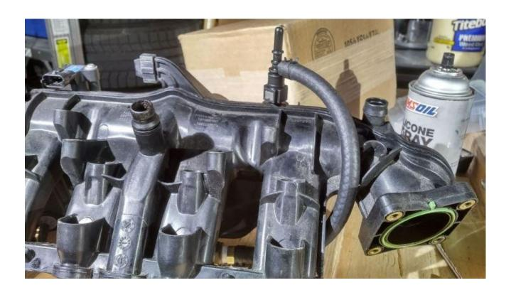
Note: The hose supplied with the kit should measure approximately 11". I measured an ideal length of 10.5" on my own intake manifold. Trim the hose if you find that it is too long.
