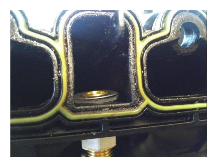
9. Slide the locknut through onto the top of the thread, and begin tightening the adapter against the thread. It may help to fit the elbow onto the adapter for this part to get more leverage. If the rubber seal starts to press out, you've tightened it too far.
