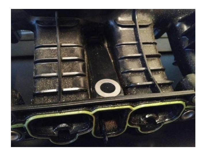
6. Using a step bit, slowly and carefully drill down to 9/16", being sure to keep it centered. If you have trouble getting it centered, you can try drilling a small 1/8" pilot hole with another drill bit first. Note that the hole on mine ended up a little too close to the opening. This is why I recommended you start further back to give you some flexibility in case this happens.
