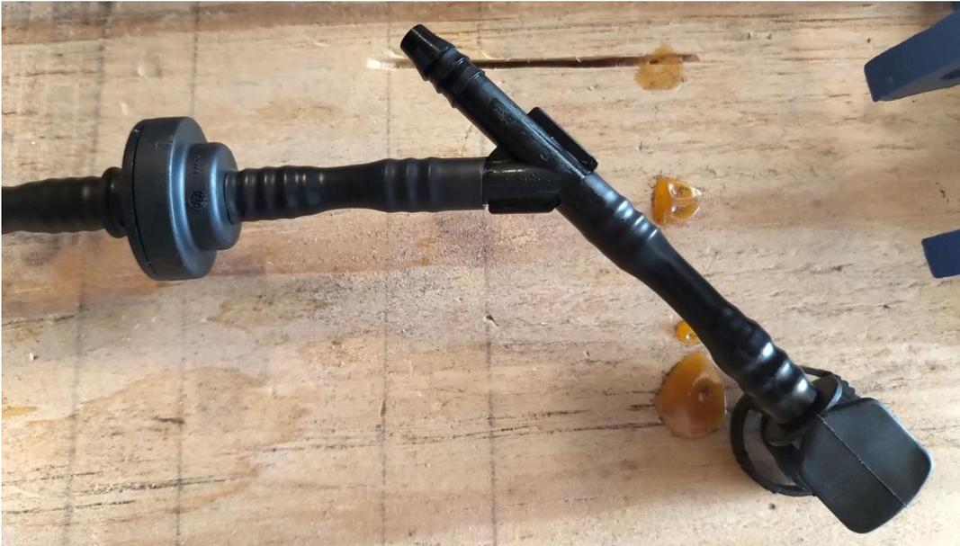
Alternately, you can use the Easy-Splice option. Cut a slit length-wise from the end of the nylon line, and use the included rubber hose and clamps to attach the Y fitting as shown below. Cut the rubber hose at 2.25", and install the longer piece on the check valve side.
